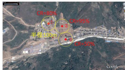
**Fig. 7 observed building collapse ratios (CRs) around the sites a01, a02, and a03**
