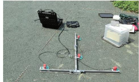
Fig.4 Observation photo a 60 cm microtremor array observation on a site at B5.
