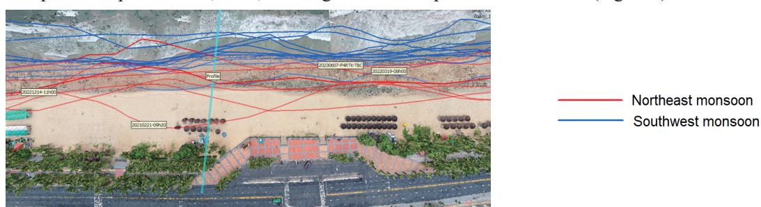
Figure 8. Extracted shorelines from UAV data
