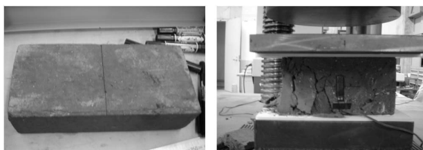
Figure 6. Masonry brick unit and compression test
