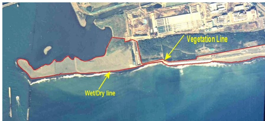
Figure 3: The wet/dry boundary is chosen as an alternative shoreline indicator which is corrected later to mean sea level (MSL)
