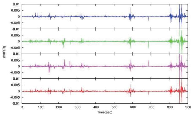
Fig.5 Velocity waveforms of 4 sensors of at observation point C11.
