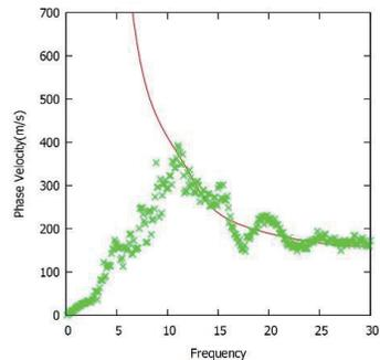
Fig.6 Phase velocity at A2. A red solid line indicates theoretical one and green crosses are observed one.
