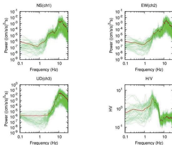
Fig.7 Power spectra and H/V spectra ratio at observation point A2. Red solid lines indicate average lines of power spectra and H/V spectra ratio and green lines are individual observed data.
