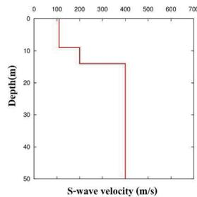
Fig.11 Estimated S-wave structure from calculating H/V Spectral ratio. A red solid line is S-wave velocity.
