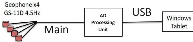
Fig.2 System of microtremor velocity observation tool GDAQ-4s that consists of geo-phone sensors, AD converting unit and Windows OS tablet.
