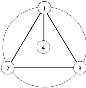
Fig.3 Triangular array setting form for miniature array. A number in small circles indicates a geo-phone sensor.
