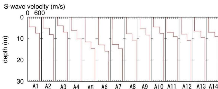
Fig.12 Distribution of S-wave structures along A-Line.
