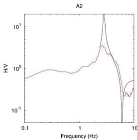
Fig.10 A red solid line is an average H/V spectral ratio and black line indicates theoretical one at A2 point.
