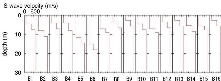
Fig.13 Distribution of S-wave structures along B-Line.
