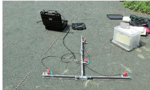
Fig.4 Observation photo a 60 cm microtremor array observation on a site at B5.
