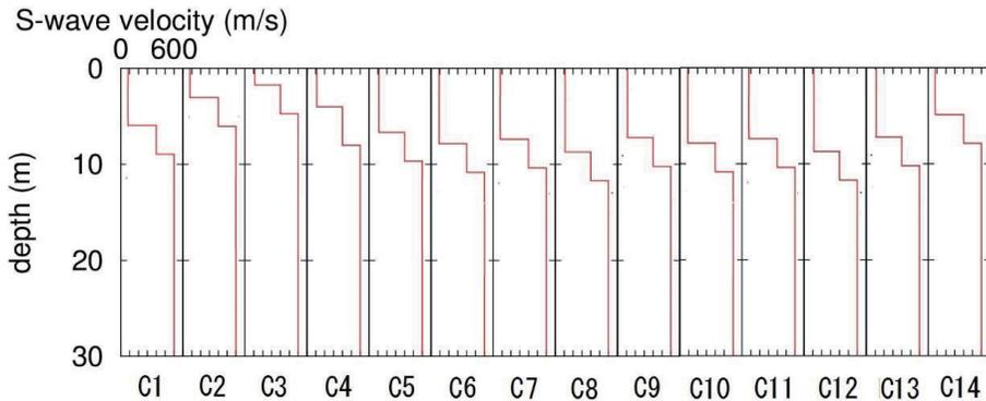
Fig.14 Distribution of S-wave structures along C-Line.
